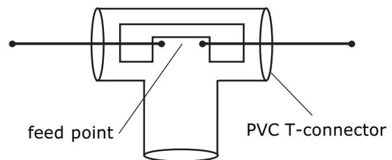
**Figure 4: Building a dipole antenna (step 3)**
