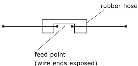
**Figure 6: Building a dipole antenna (step 5)**
