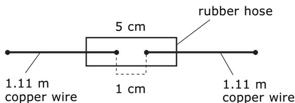
**Figure 5: Building a dipole antenna (step 4)**
