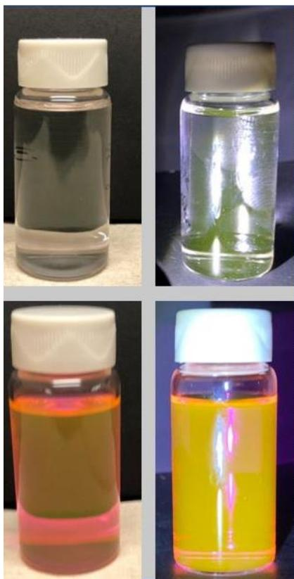
**Figure S-2.** Orange highlighter extract solution (top across); pink highlighter extract (bottom across). Pictures on the right-hand side are illuminated in a light box. The pink highlighter solution (bottom right) is highly fluorescent; the orange highlighter solution (top right) is not.
