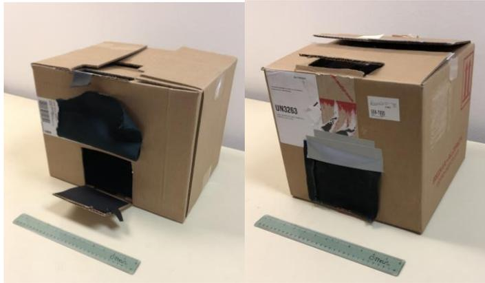
**Figure S-3.** Two light box models of varying size and modifications are shown. Any box with an adequately spacious and dark interior should suffice.
