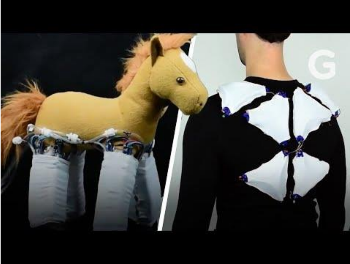
Pneumatic textile back brace
