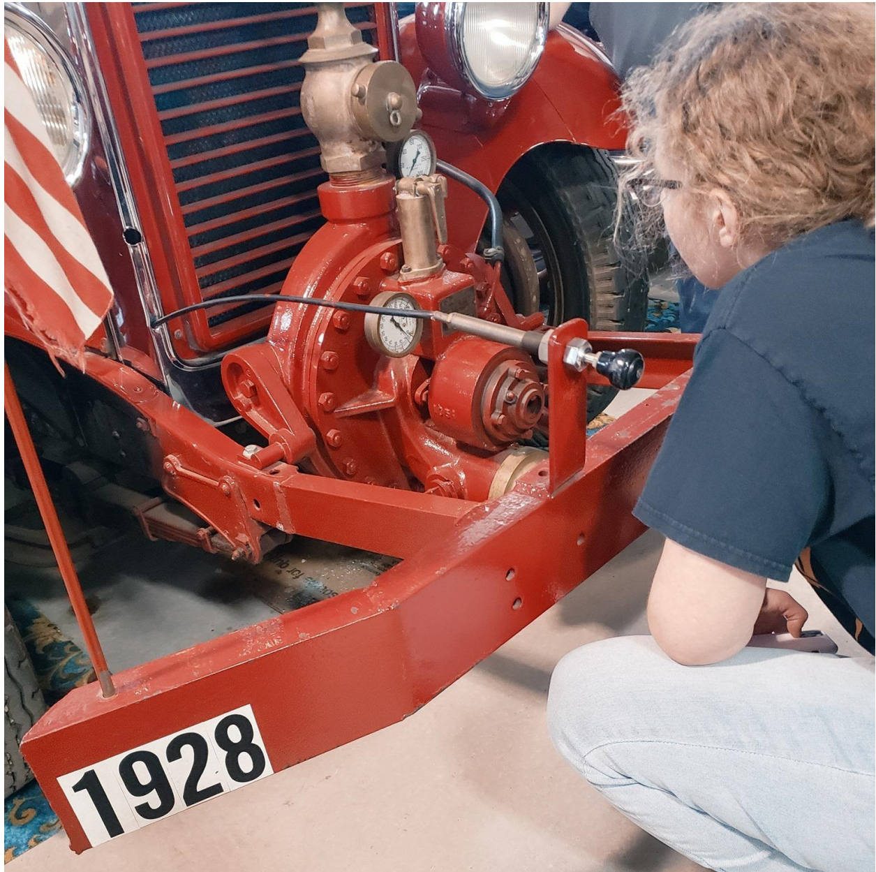
Figure 16. Science research student studying the governor on the fire truck, which malfunctioned while fighting the fire. Artifact from O'Fallon Historical Museum.
