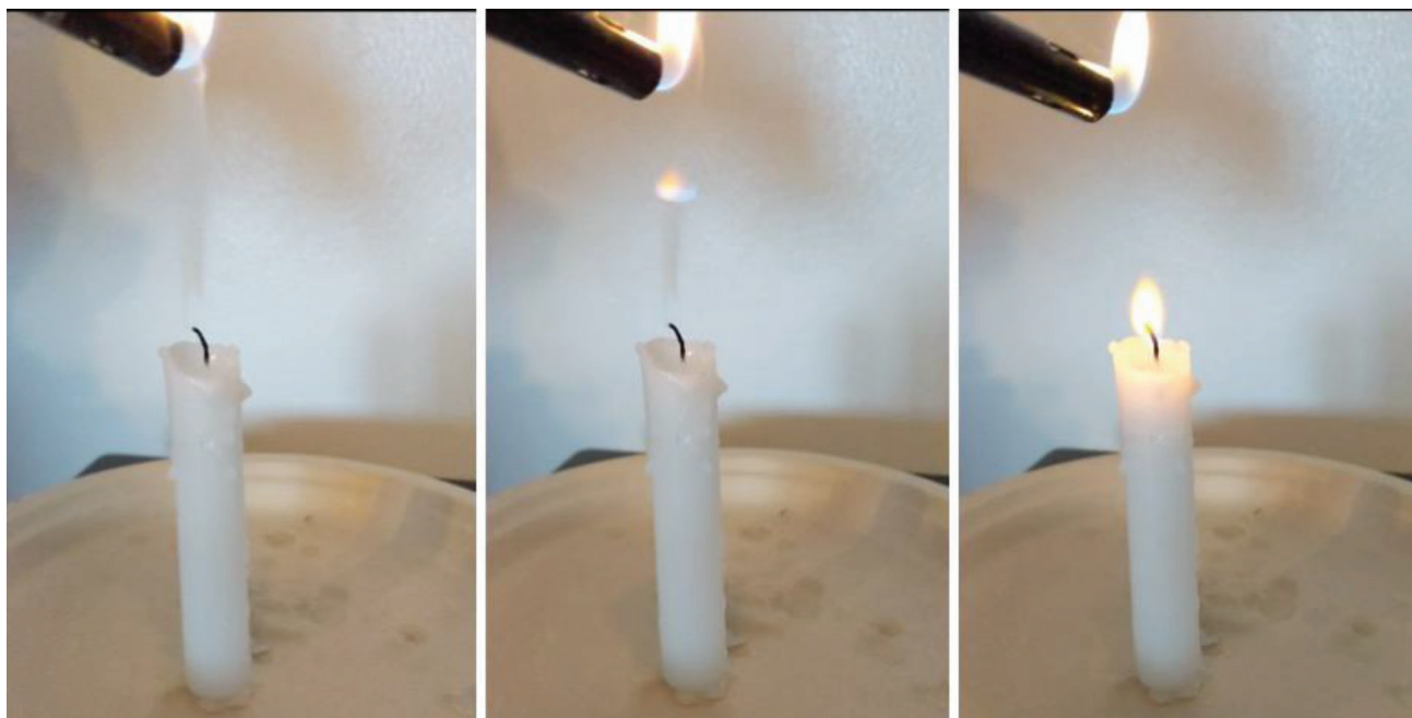
FIGURE 2: By placing a lighter flame into the plume of smoke [evaporated hydrocarbons] coming from a recently extinguished candle, a flame can be made to “jump” down the column of smoke and relight the candle [full video of this process is available in Resources].
