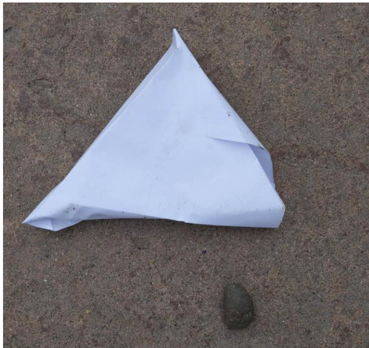
Figure 2. A protect-the-Pringle structure is dropped from waist height to the floor.
